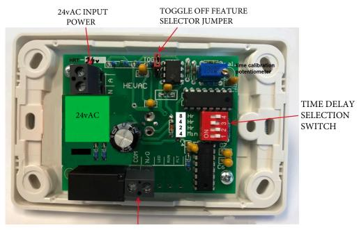
VOLTAGE FREE RELAY SPST CONTACTS rated @ max 5A (res.)(2A Ind.)
