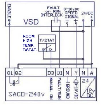
NOTE: TERMINALS M & N INTERNALLY CONNECTED
