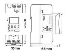
Advanced pre-setting one week before Digital electronic time switch with daily programs Repeat programs with 16 on/off setting: and manual over-ride Lithium battry power reserve Auto time error correction ± 60sec, weekly
