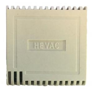
The SRTAAA-D is an averaging type room sensor to be used in groups of 3 (wired in parallel). It is intended for use with Hevac brand HTC 3, 5 and Digital series controllers. The sensor has a NTC characteristic (increase in temperature = decrease in resistance) and changes approximately 240 ohms per degree.
