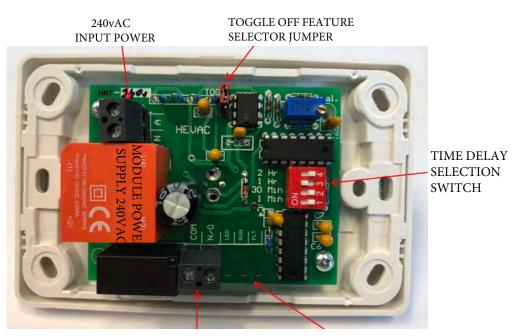
VOLTAGE FREE RELAY SPST CONTACTS rated @ max 8A (res.)(2A Ind.)
