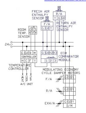
TEMPERATURE CONTROL SYSTEM WITH MODULATING ECONOMY CYCLE O/P USING ECM MODULE FOR F/A-R/A ENTHALPY COMPARATOR INHIBIT INTERLOCK
