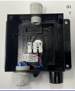
24 Volt Supply Active DC 4-20mA DC Signal Out
