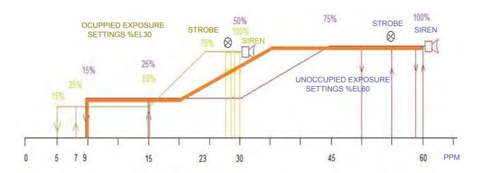
NOTE: THE CODE ALSO CALLS UP FORCED RUNNING OF THE FAN SYSTEM TO MEET MINIMUM VENTILATION REQUIREMENTS IN A 24HR PERIOD. AS SUCH THE HCP7 INCLUDES AN IDLE TIMER THAT TRIGGERS FAN OPERATION FOR 10 MINUTES (ADJUSTABLE) IF THE FAN SYSTEM HASNT STARTED IN THE PREVIOUS 24HRS (ADJUSTABLE).
