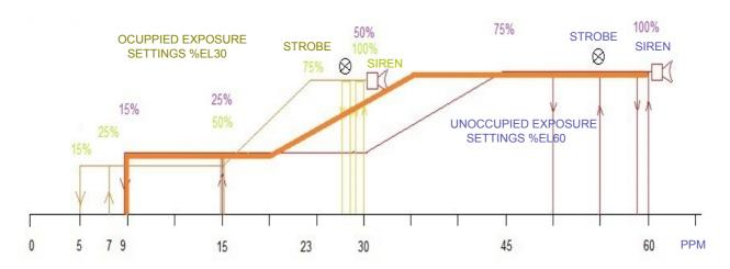
NOTE: THE CODE ALSO CALLS UP FORCED RUNNING OF THE FAN SYSTEM TO MEET MINIMUM VENTILATION REQUIREMENTS IN A 24HR PERIOD. AS SUCH THE HCPT INCLUDES AN IDLE TIMER THAT TRIGGERS FAN OPERATION FOR 10 MINUTES (ADJUSTABLE) IF THE FAN SYSTEM HASNT STARTED IN THE PREVIOUS 24HRS (ADJUSTABLE).
