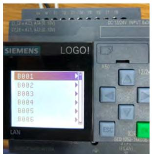
SCROLL DOWN THE PARAMETER LIST USING THE **DOWN** BUTTON TO THE LOGIC BLOCK THAT NEEDS EDITING . SEE ATTACHED LIST OF LOGIC BLOCKS WITH PARTICULAR SETTINGS THAT MAY NEED ADJUSTING TO SUIT SITE CONDITIONS ETC.
