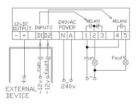
EXAMPLE CONNECTION WHEN EXTERNAL 12vDC POWER IS AVAILABLE FOR NWIF INPUTS
