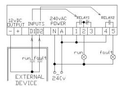
EXAMPLE CONNECTION WHEN NO EXTERNAL 12vDC POWER AVAILABLE FOR NWIF INPUTS
