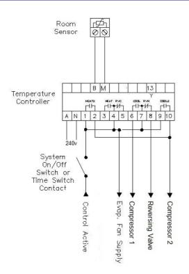
Typical for Compressor Reversing Valve type A/C Units where the R/V energises on Heating
