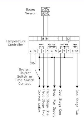
Typical for Heat/Cool type Air-conditioning Units
