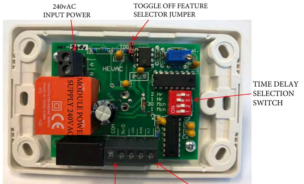
VOLTAGE FREE RELAY SPST CONTACTS rated @ max 8A (res.)(2A Ind.)
