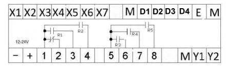
12-24 Volt Supply Neutral 5 Relay 3,4 & 5 Common (internally connected to terminals M) 6 Relay 3 Normally Open + 12-24 Volt AC or DC Supply Active 7 Relay 4 Normally Open Relay 1 & 2 Common Relay 5 Normally Open (FAN) Relay 1 Normally Closed Μ Signal ground 3 Relay 1 Normally Open Analog Modulating Output 0-10 vDC
