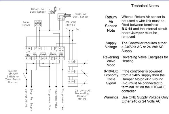
Typical for Compressor Reversing Valve type A/C Units where the R/V energises on Heating
