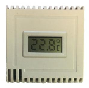
The SRTA-DLCD is an averaging type room sensor complete with LCD temperature display to be used in pairs (wired in parallel). It is intended for use with Hevac brand HTC 3, 5 and Digital series controllers. The sensor has a NTC characteristic (increase in temperature = decrease in resistance) and changes approximately 160 ohms per degree.
