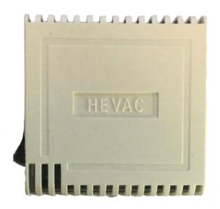
The SRT-DB is a room sensor complete with system on/off and after hours run switch functions. It is intended for use with HTC-Digital-LCD. The sensor has a NTC characteristic (increase in temperature = decrease in resistance) and changes approximately 80 ohms per degree.
