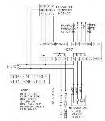
Application Example (2) 4 X HEVAC CO SENSORS & 2 X HEVAC NO2 SENSORS c/w MODULATING VSD OUTPUT
